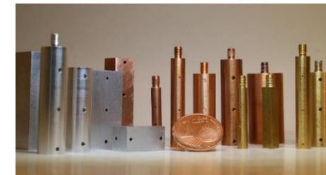
selection of available test heads
