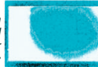
Delamination in sintered power module
