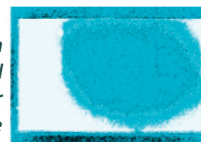
Delamination in sintered power module
